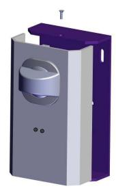
Carefully clip the back cover into the correct position.
