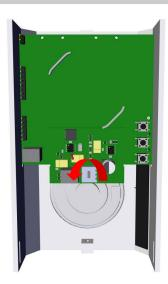
Insert a terminal screwdriver in the Pot and rotate as follows:
